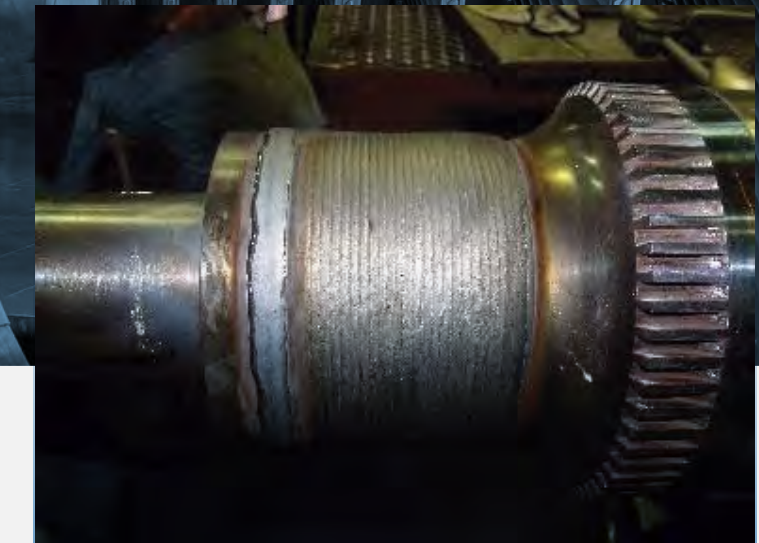
• Auto-TIG Shaft Repair
